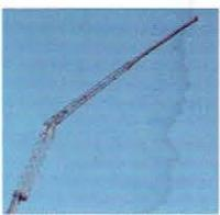
A bi-fold swingaway lattice extension easily stows on the side of the base boom for easy transport. The choice of a manual or optional hydraulically offsettable extension is available. To take it even further, up to two additional extension inserts can be added to provide up to 237 ft. of tip height.
