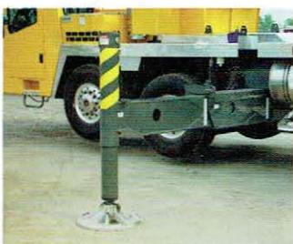
Two-stage inverted jack outriggers provide 3 position settings – 0%, 50% and 100%.
