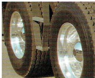
Front and rear air over walking beam suspension provides a smooth ride at 65 mph. Aluminum wheels, fenders and decking are also standard features.
