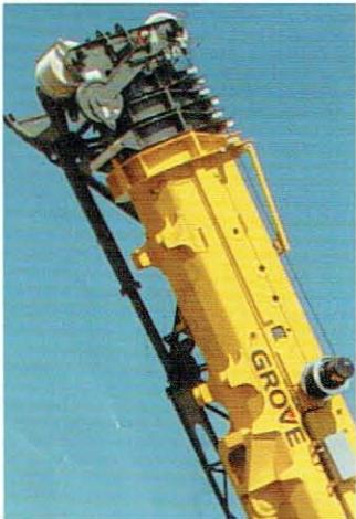
The superstructure features a full power five section MEGAFORM boom that can reach to a maximum tip height of 150 ft. The TWIN-LOCK boom pinning system provides pre-selection of boom extension modes to efficiently pin boom sections automatically.
