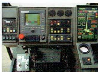
Crane functions are controlled by ECOS (Electronic Crane Operating System) with CAN-BUS. The EKS4 load moment indicator provides detailed feedback and control of the cranes operating functions.
